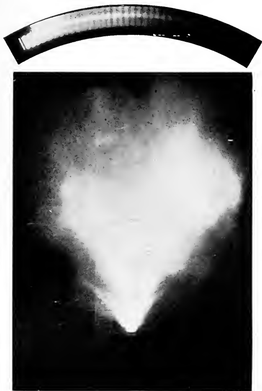
FIG. 133. Flame from Kieselguhr Dynamite
